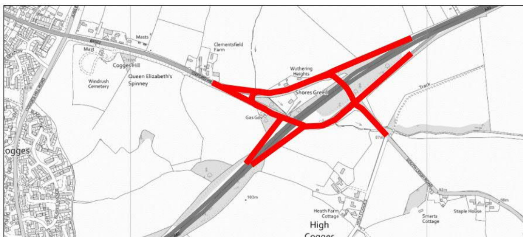
Figure 40: Option 2D: West facing slip roads at Shores Green - grade separated
