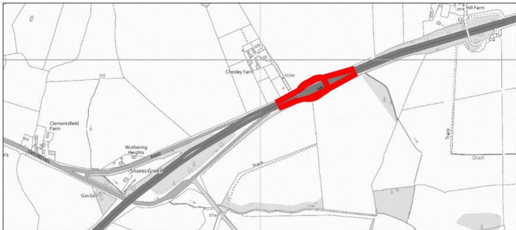
Figure 43: Option 4B: Half or full roundabout on the A40 to the east of Shores Green
