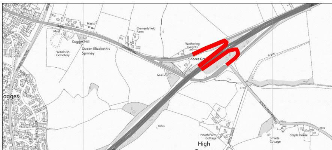
Figure 39: Option 2C: West facing slip roads at Shores Green – D-Link alternative arrangement
