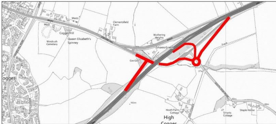
Figure 38: Option 2B: West facing slip roads at Shores Green - alternative arrangement
